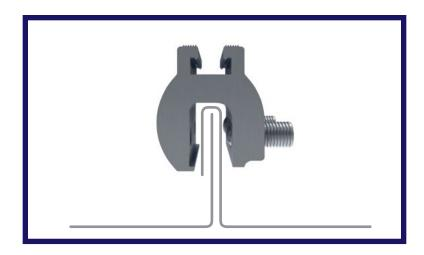
Position SimpleBlock assembly on the panel seam. Make sure the block is fully seated on the metal seam.
