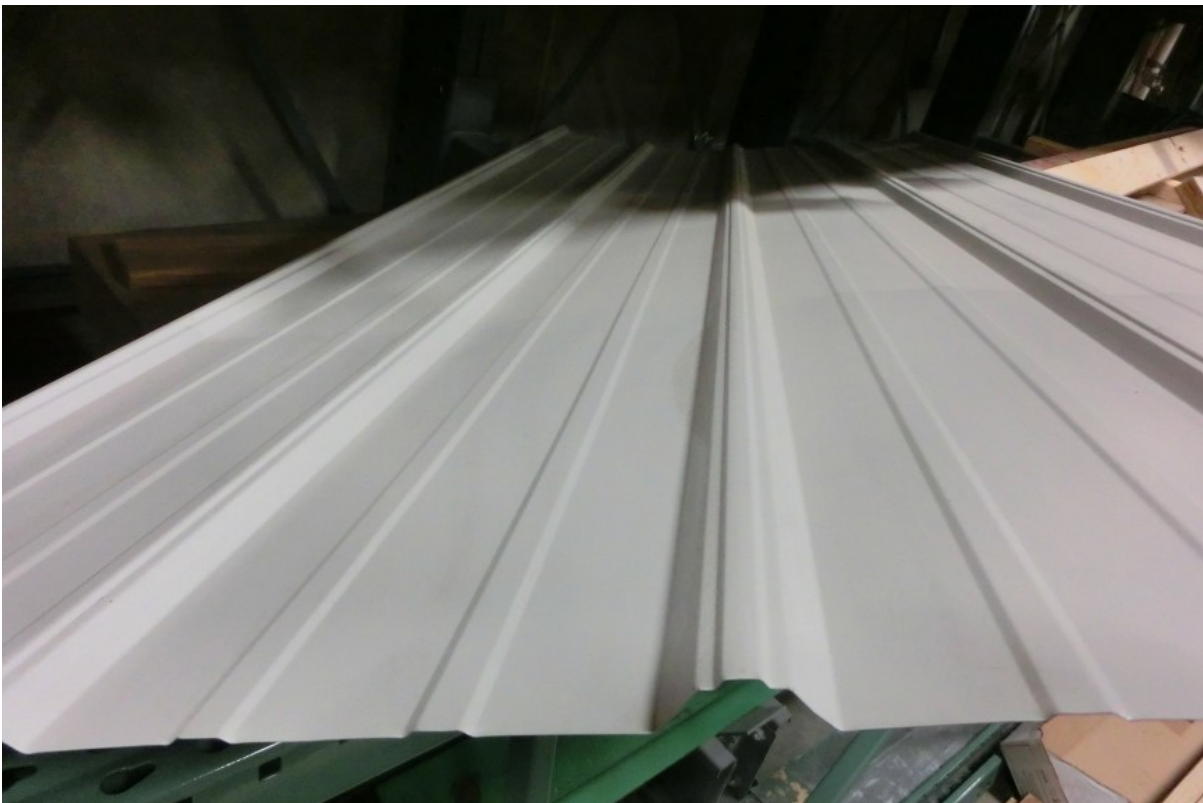
Photo 2: Metal Roofing Used for Test (27 Gauge)
