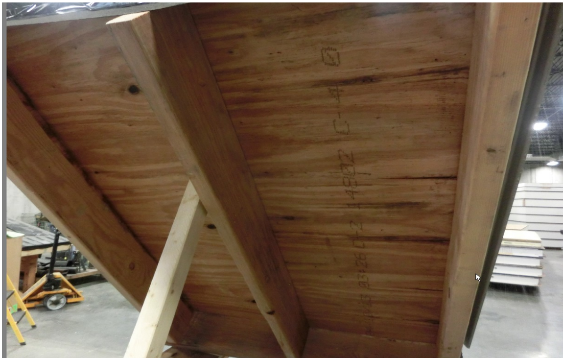
Photo 6: Underside of Roof Deck After Rain Test
