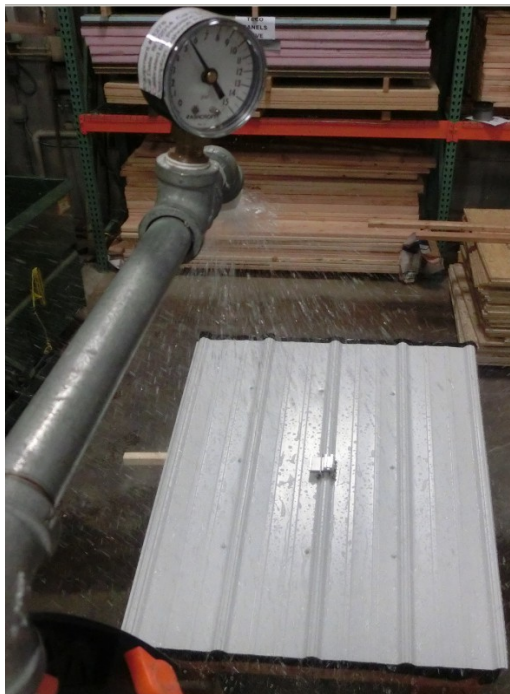
Photo 4: Spray Test of Roof Deck at 3:12 Pitch
