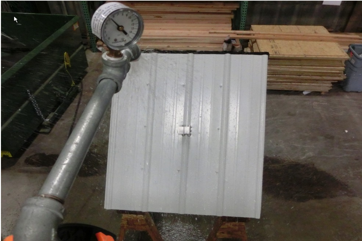
Photo 3: Spray Test of Roof Deck at 12:12 Pitch
