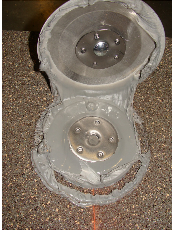
Photo 7: Typical Failure in Lateral Load Test
