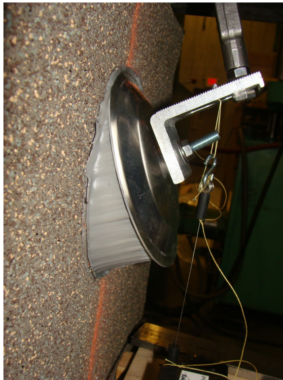
Photo 8: Typical Failure in Lateral Load Test
