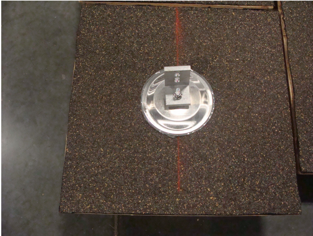
Photo 3: Test Deck Sample with SimpleGrip Assembly
