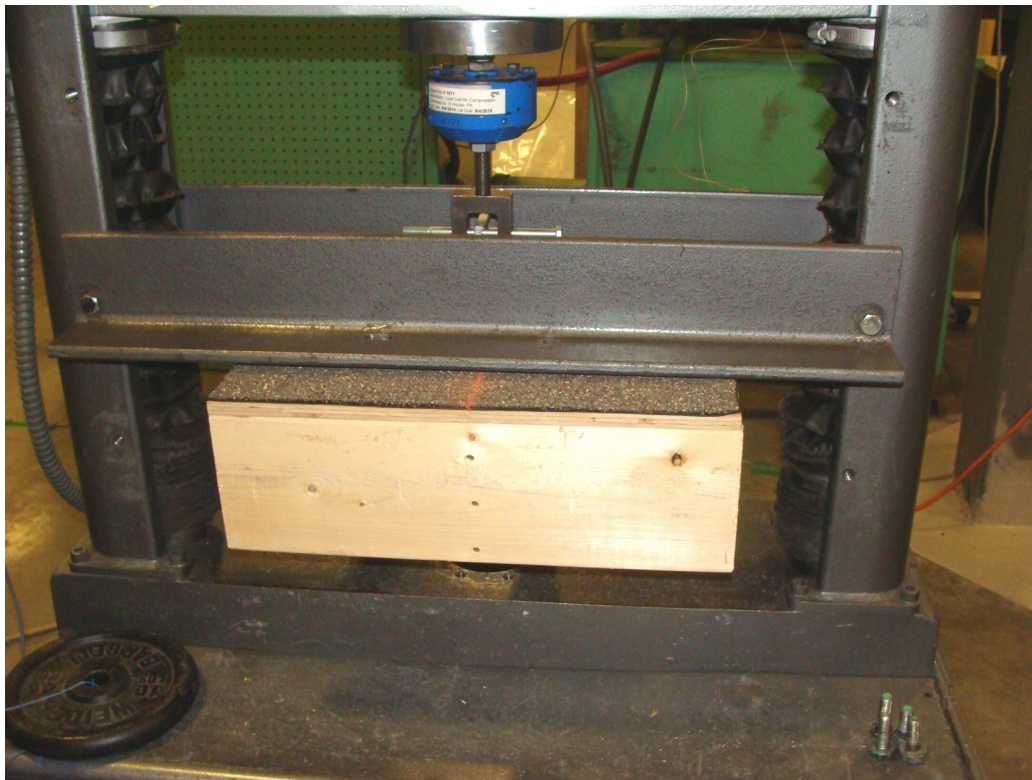
Photo 4: Typical Uplift Load Test Setup
