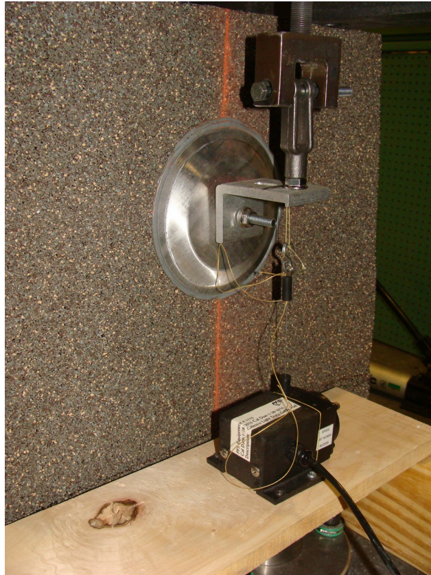
Photo 5: Typical Lateral Load Test Setup
