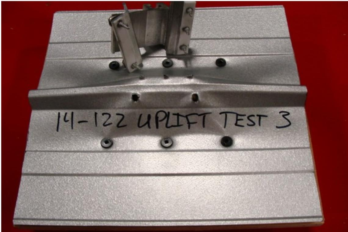
Photo 6: Typical failure in uplift load test (26 Gauge)
