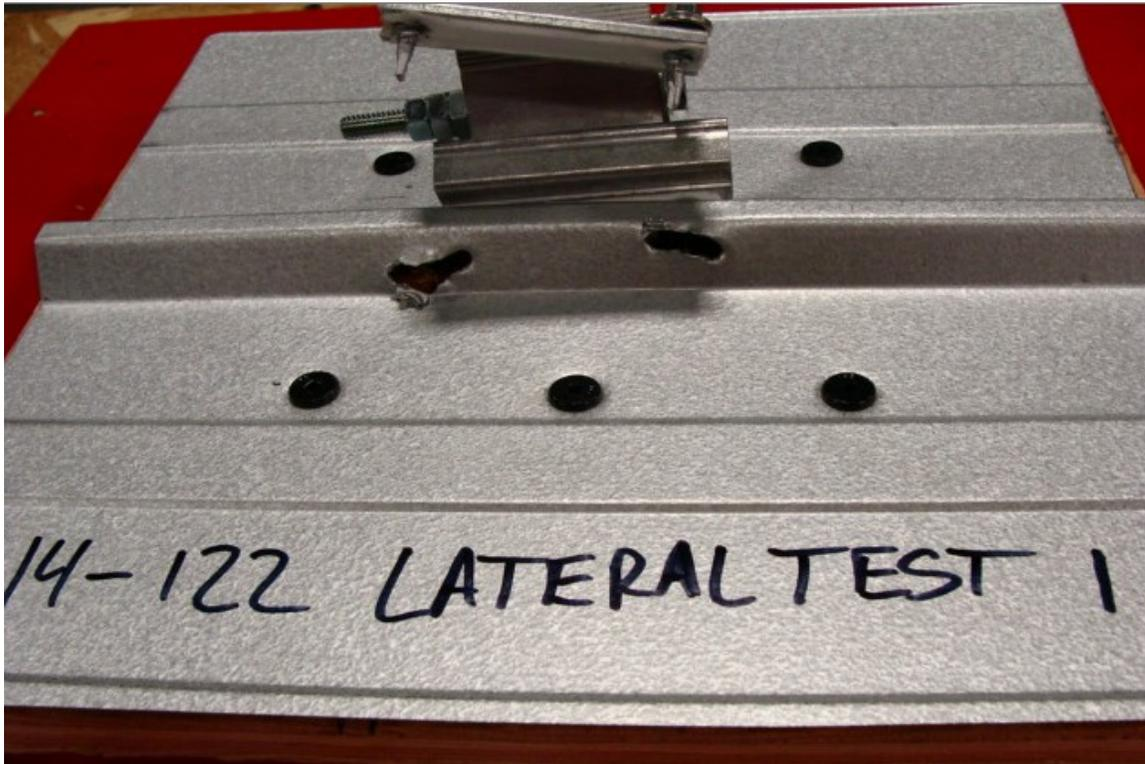
**Photo 7: Typical failure in lateral load test (26 Gauge)**
