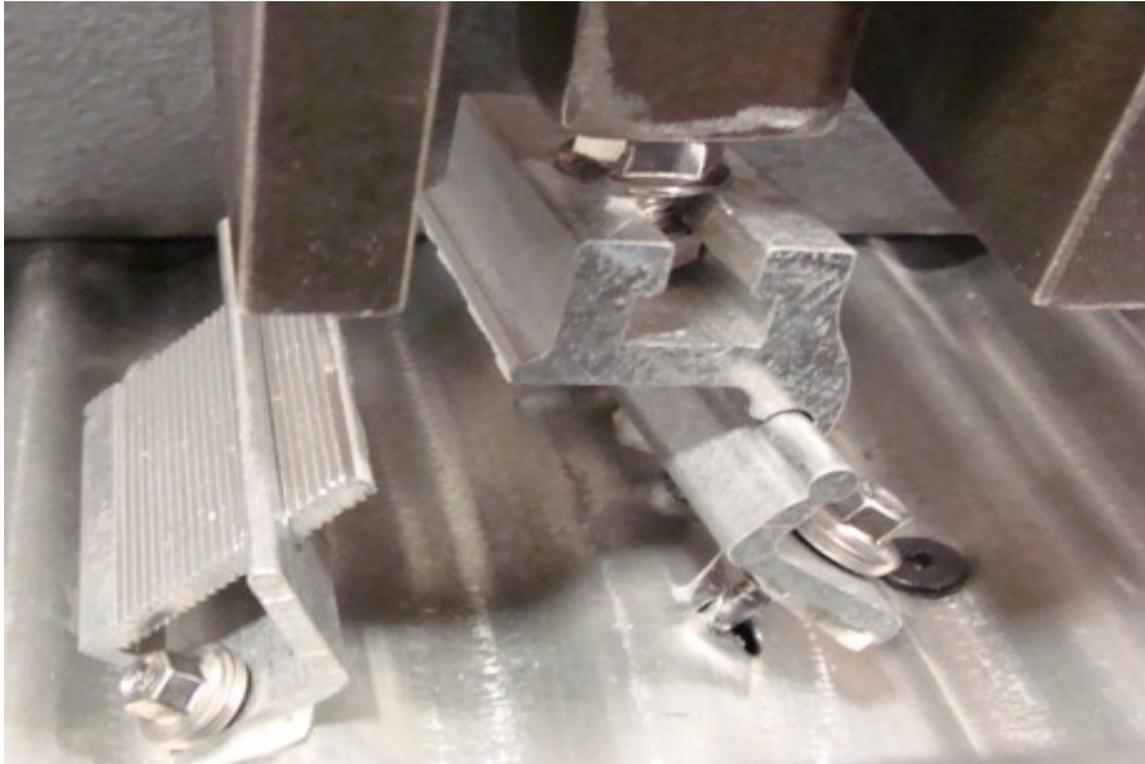
**Photo 9: Typical failure in uplift load test (24 Gauge)**
