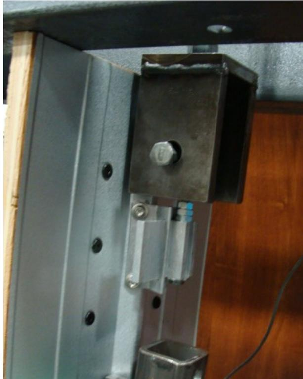
Photo 5: Typical lateral load test setup
