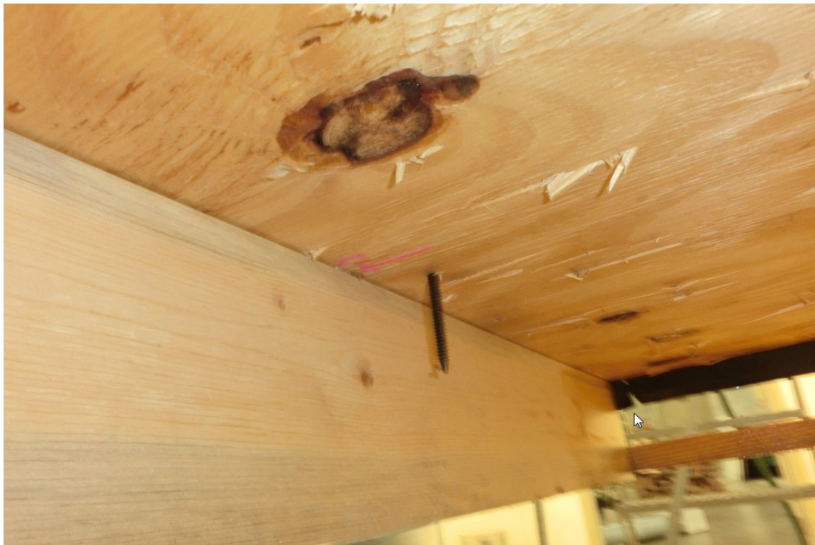
Photo 10: Underside of the Test Deck After Rain Test
