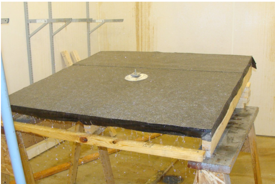
Photo 4: Test Deck Sample at 2:12 Pitch
