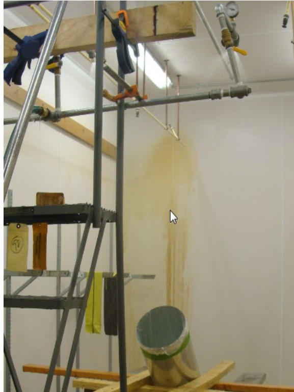
Photo 3: Rain Test Calibration Setup
