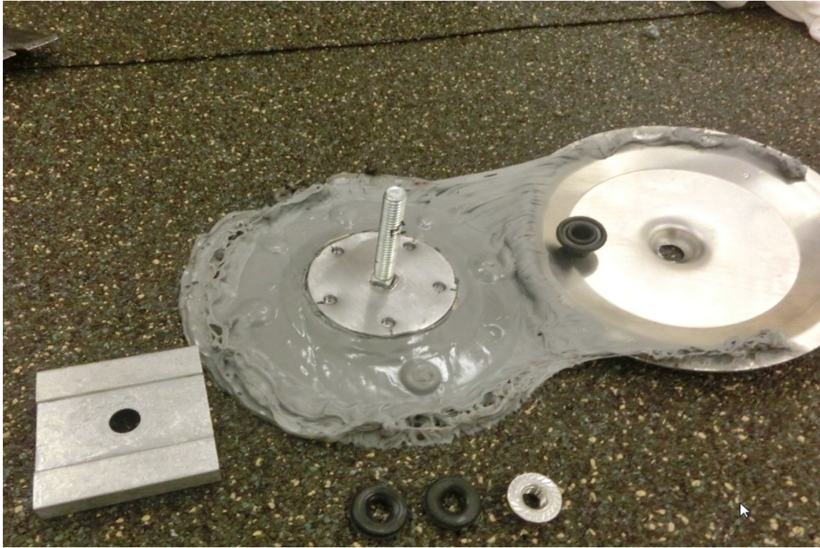
Photo 9: Top Surface of Test Deck After Rain Test, Compression Plate Removed
