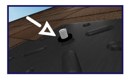
After the flashing is in place, install the EPDM washer over the stud.
