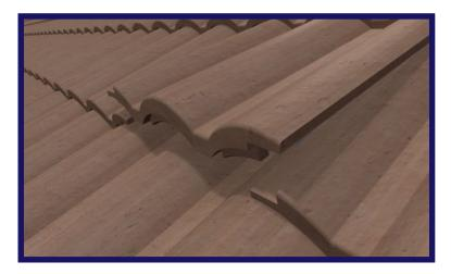
Lift up the tile above which overlaps the Tile you want to run conduit across. The tile does not need to be removed, just lifted on the front edge.
