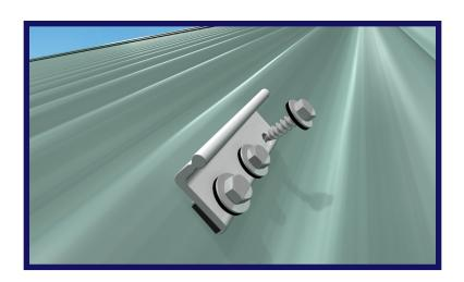
Pre-installation note: Check one complete CorruSlide assembly on the roof panel for proper fit and mounting location prior to installing the scews.
