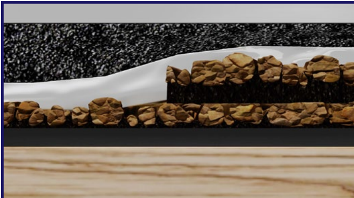
A layer of flexible foam pushes the sealant deep into the shingle's granules and around shingle steps
