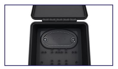
Using a pilot drill, begin drilling out the box at the desired conduit pass through location. It is acceptable to use any location inside the watertight oval for a penetration. Drill through both the box and into the roofing, marking the location on the roof of the clearance hole, transferring the proper drill location to the roof surface.
