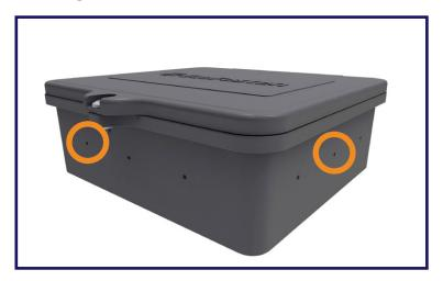
Prior to installation, use a step drill bit to place pass through holes for conduits or water-tight connectors. Drill bit starter locations are provided on the sides and front of enclosure. Do not install conduit facing up roof.
