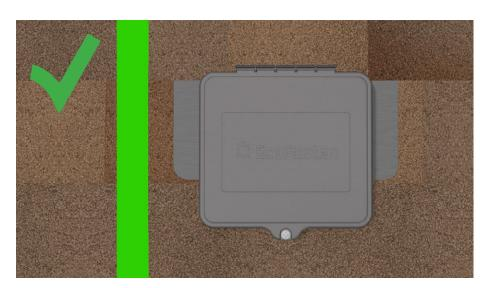
Do not install over a rafter when using the pass-through.
