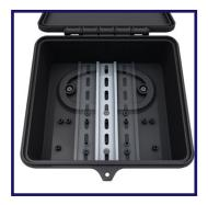
Install DIN 3 rail at preferred location using hardware provided. Up to 6 7/8" long DIN 3 rail can be installed in one horizontal orientation and three vertical options within the box using the provided #8x3/8" Phillips head screws.
