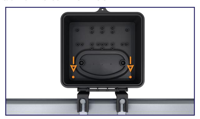
When installing the junction box on the uproof side of the rail, two 1/8" field drilled weep holes must be installed in the downslope corners of the box.
