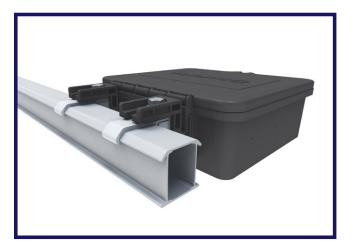
Use ClickFit MLPE Mount to attach Rail Connectors to rail. Ensure junction box is pushed as close to the rail as possible. Torque to 80 in-lbs, do not over-tighten. If installing in areas with ground snow loads greater than 40 psf, install Junction Box directly next to module frame edge.
