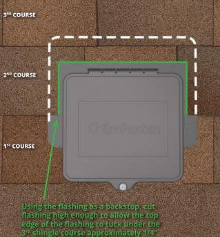
In summary, to avoid an exposed and un-flashed shingle butt-seam or keyway, the installer can cut away a section of the 2nd shingle course to allow the flashing to tuck up under the 3rd course. This flashes any exposed shingle butt-seam or keyway. As an extra layer of protection, run a bead of roof sealant between the flashing and 2nd shingle course just inside the cut line.
