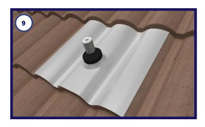
9. Install the tile-level flashing. It is possible to use the 18 x 18" flashing or other third party cone flashing. EcoFasten's 18 x 18" flashing is malleable, so it is possible to shape the flashing to conform to the shape of the tiles.
