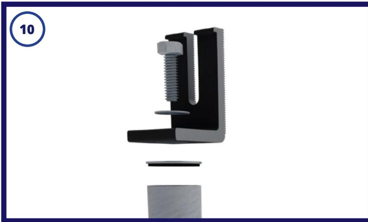
10. Install desired bracket or L-Foot using the included racking hardware. Take care to install 1-1/4" bonded sealing washer directly to the top of the post to keep out water. Install the L-foot to the top of this washer.
