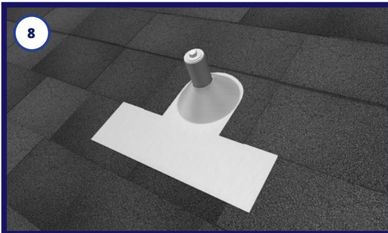
8. Allow roofing to proceed to next shingle course. Use a hooked blade to cut a space out of the shingle that overlays the flashing around the flashing cone.
