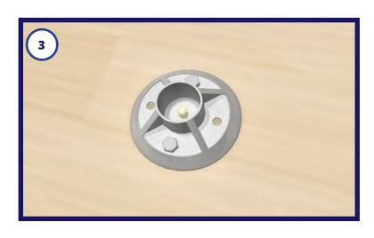
3. Backfill pilot holes with a sealant compatible with the roofing material. Insert the grade-8 cap screw through the hex slot on bottom of the QB-1 Base. Place QB-1 Base over drilled pilot holes and secure fasteners in place to a solid, snug fit.
