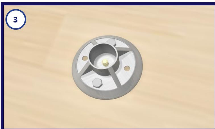
3. Backfill pilot holes with a sealant compatible with the roofing material. Insert the grade-8 cap screw through the hex slot on bottom of the QB-1 Base. Place QB-1 Base over drilled pilot holes and secure fasteners in place to a solid, snug fit.
