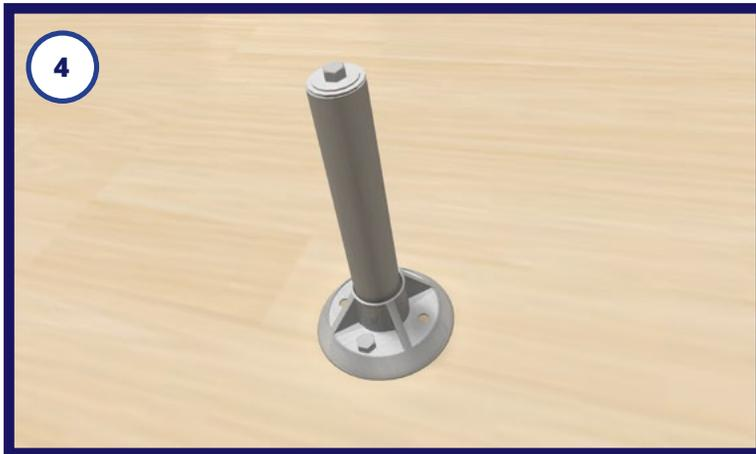
4. Secure post to QB-1 Base by completely screwing post into captive grade-8 cap screw. Install racking hardware to seal off the top of the post.
