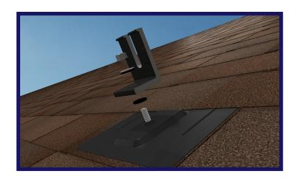
Place the bare EPDM washer over the stud, pushing it all the way down. Then place an EcoFasten compression bracket over the stud and bare EPDM washer, followed by the bonded sealing washer with the rubber side facing down.
