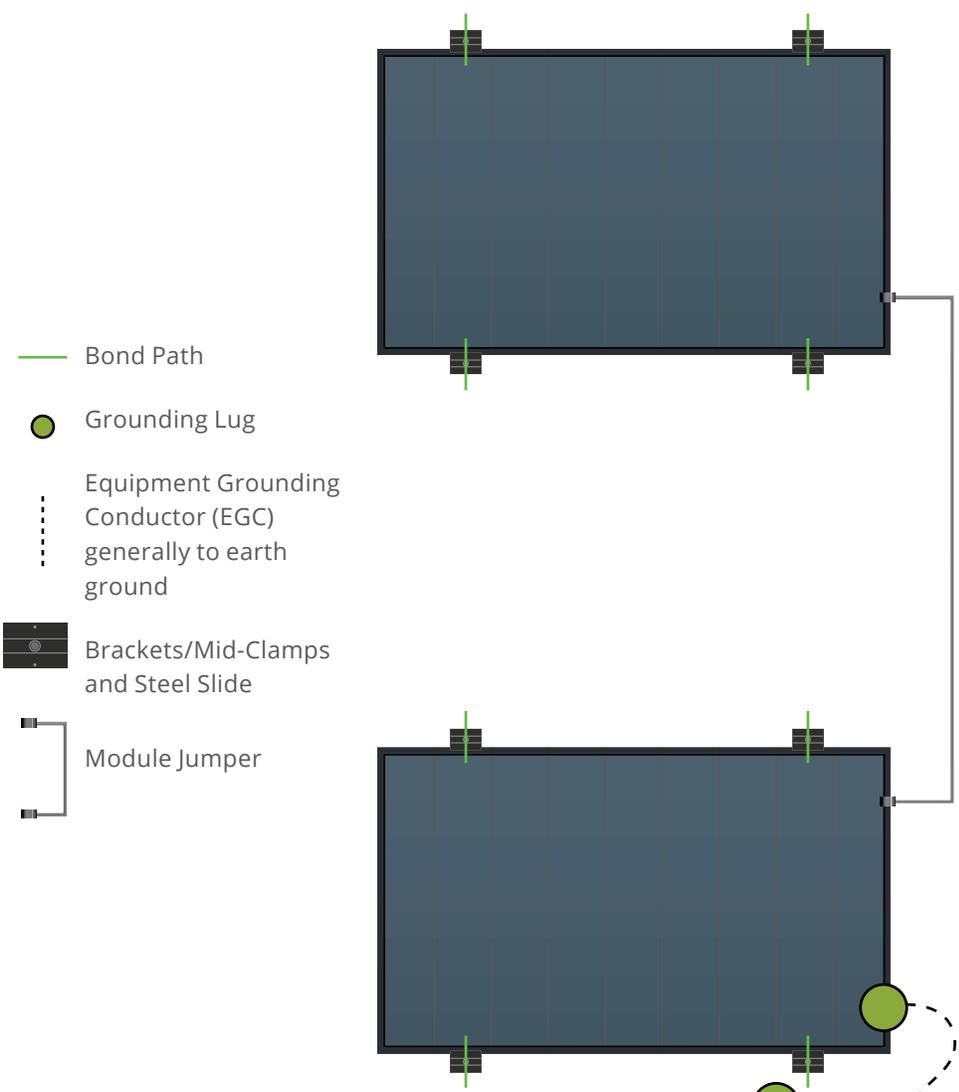
Ilco SGB-4 Approved for Mounting to Steel Slide as alternate grounding location
