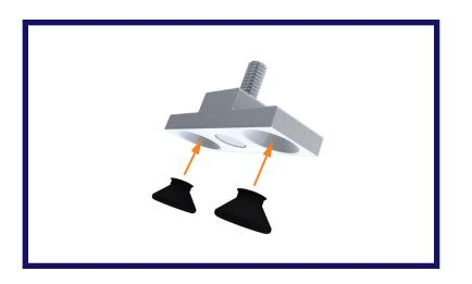
Preinstall both cone-shaped rubber SimpleSeal bushing into the SimSupport bracket by inserting the tip of each cone in to the corresponding shape in the bottom of the compression bracket. The ridge around the tip of the cone will hold the bushing in place until the bracket is installed.
