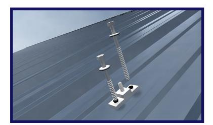
Thread the 5/16" EPDM bonded sealing washers onto the 5/16" lag bolts and insert the bolts into the top of SimpleSeal bushings.
