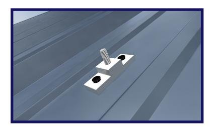
Place the compression bracket on roof surface above a supporting structural component, ensuring that the bushing sits flat against the roof surface.
