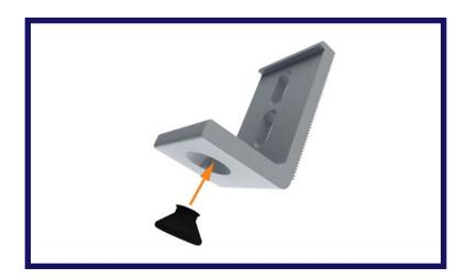
Pre-install the cone-shaped rubber Sim Seal bushing into an EcoFasten compression bracket of your choice prior to installation by inserting the tip of the cone into the corresponding shape in the bottom of the compression bracket. The ridge around the tip of the cone will hold the bushing in place until the bracket is installed.
