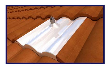
Replace any additional tiles that were removed adjacent to the location of the tile to be replaced, then place the tile replacement flashing over the post and mount, allowing flashing to interlock with surrounding tiles properly. Secure the post by tightening it down using a pair of channel lock pliers. Replace surrounding tiles.
