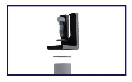
Install desired bracket or L-Foot using the included racking hardware. Take care to install 1-1/4" bonded sealing washer directly to the top of the post to keep out water. Install the L-foot to the top of this washer.
