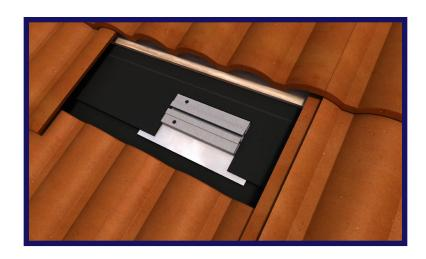
Waterproof at underlayment level according to roofing manufacturer instructions and Tile Roofing Institute Guidelines. Alternative Flashing Methods may be approved by the AHJ at their discretion.
