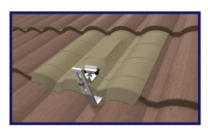
Replace the removed tile with appropriate shaped Tile Hook Flashing. It is permissible to nail the flashing to the batten using 1-2 nails as seen fit to prevent the flashing from moving.
