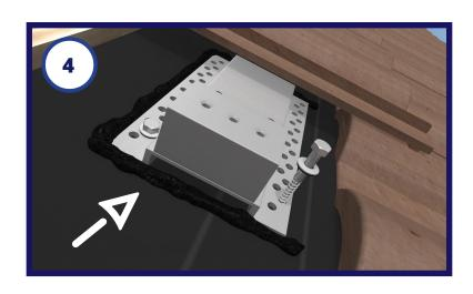
4. Place a bead of caulk around the base plate leaving the bottom edge exposed. Then install the base plate using the two 5/16" x 4" lag bolts w/ bonded washers included in the packaging.
