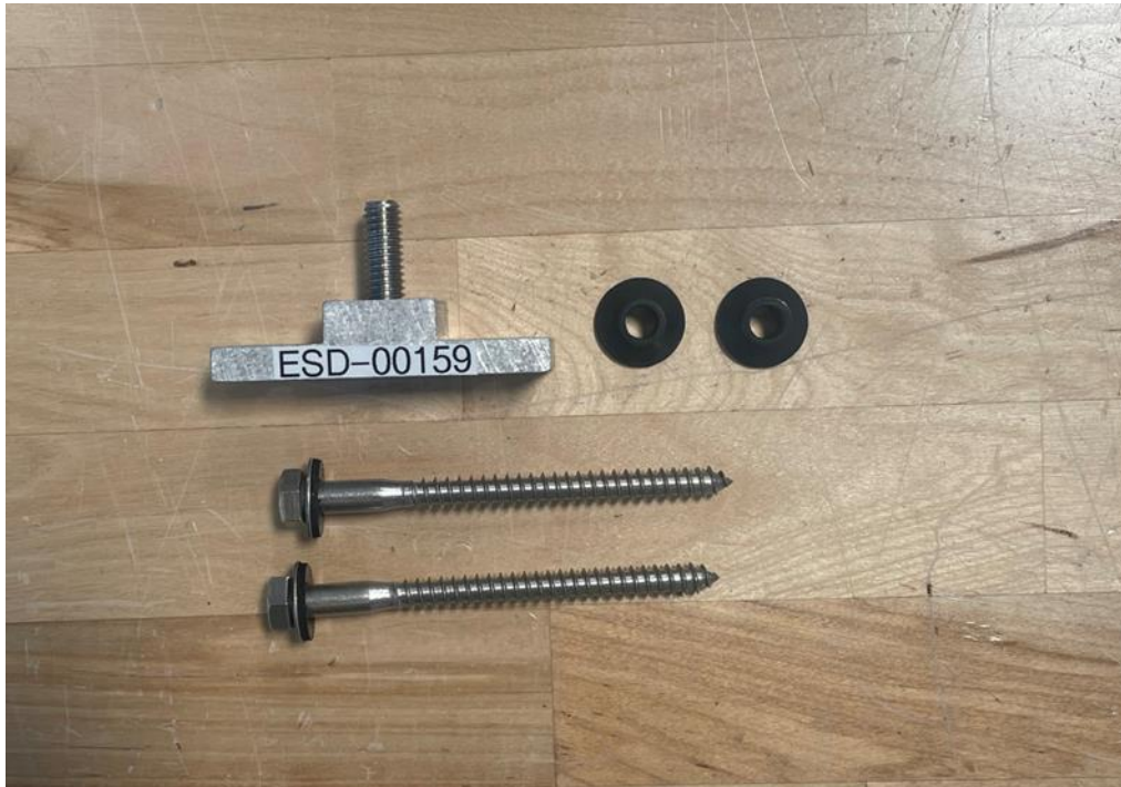
Photo No. 1 Unassembled Test Specimen
