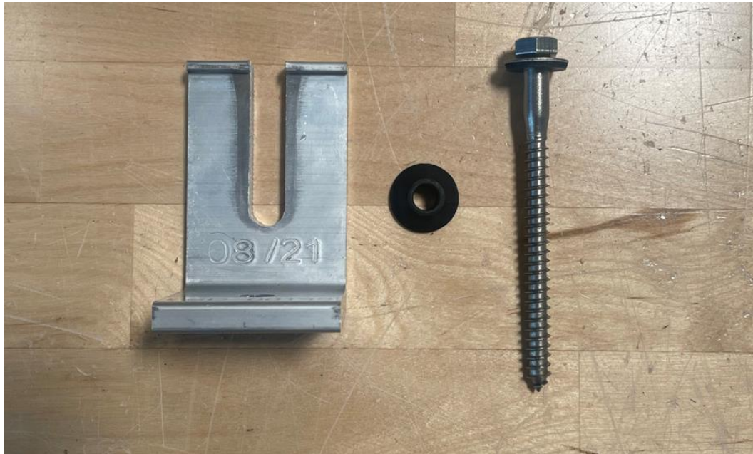
Photo No. 1 Unassembled Test Specimen
