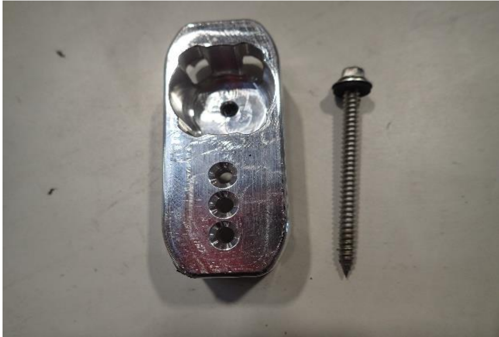
Photo No. 1 Unassembled Test Specimen
