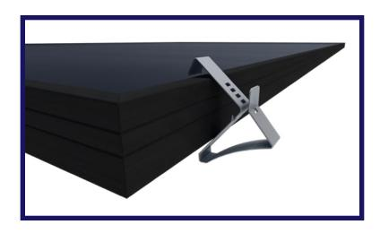
Use the properly sized Side Clip for the module frame thickness. Place the Side Clip on the side edge of the module frame, with the hook's top portion resting on the top edge of the frame.
