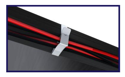
Place the wires inside the Side Clip. Secure up to four (4) 10AWG wires or up to six (6) 14AWG or equivalent bundled diameter wires inside the Side Clip.
